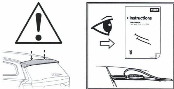
**EN** If plastic spoiler is in the area where upper hooks will be mounted, always use the spoiler kit with the reinforcement strap, according to separate instruction for **Plastic Spoiler Reinforcement Strap**.
