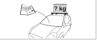
When these roof racks are to be used on a vehicle that is driven off sealed roads, the manufacturer maximum roof load rating (to be found in the vehicles User Manual) should be *divided by 1.5.* Do not forget to subtract the complete crossbar system weight from your maximum carrying capacity.
