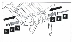
6. Replace the assembly pieces and tighten with **T1** 6mm Allen Key and **T3** 13mm Socket Wrench.
