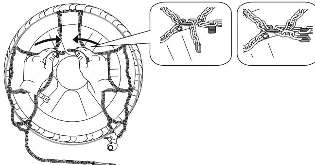
**EN** Each snow chain can fit several tyre sizes. It may happen that an adjustment of the snow chain dimension might be required in order to perfectly fit the tyre. This adjustment can be done using the adjusting links on the upper side chain.
