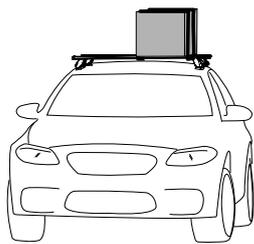
**60kg load rating** (Urban road) = **30kg load rating** (Off road - 60kg / 2)
