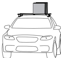
$$60\text{kg load rating (Urban road)} = 30\text{kg load rating (Off road - } 60\text{kg} / 2)$$
