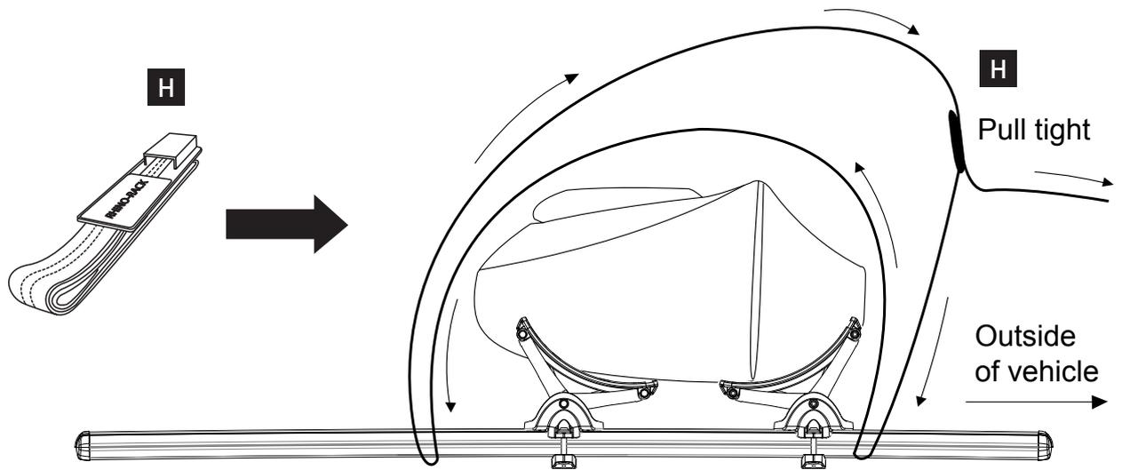
**8** Loop the straps under the crossbar as shown
